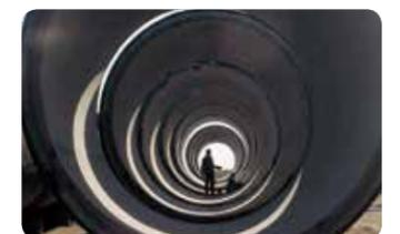
Pre-stressed Concrete Cylinder Pipe
